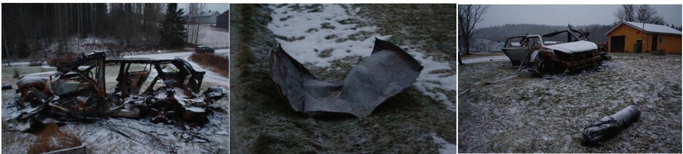
The explosion blew away the roof of the car and it landed approx. 1 meter from one firefighter
